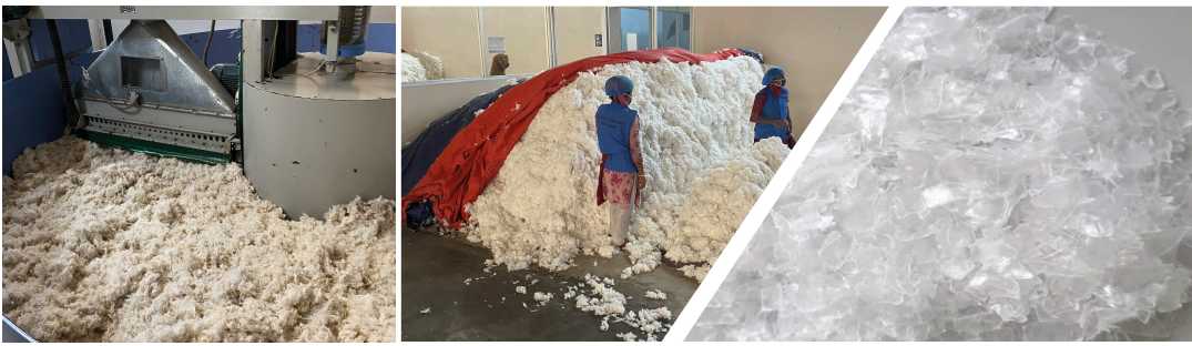
The cotton is then cut down into short fibres and processed to check for impurities.
